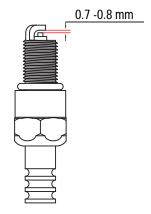
Standard Spark Plug: E6TC/E6RTC/BPR7HS
