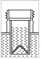
Do not overfill the fuel tank. Provide space for fuel expansion.
